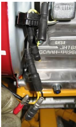
1 DISCONNECT THE BLACK WIRE FROM THE SPARK
