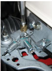
3 ATTACH THE THROTTLE SIRGA
