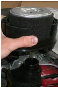
2 REMOVE THE AIR FILTER
