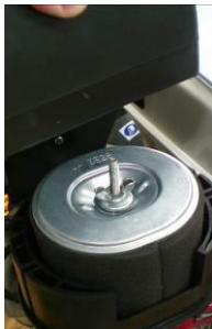
1 REMOVE THE AIR FILTER COVER
