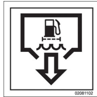
Drain outlet for fuel filter water sump
