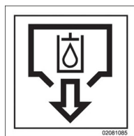
Hydraulic oil reservoir outlet
