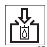
Hydraulic oil reservoir inlet
