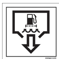
Water sump fuel filter outlet
